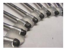
Allow the glue to set overnight. Then turn the disk over and apply a generous amount of glue to firmly seat the rods on the disk.
