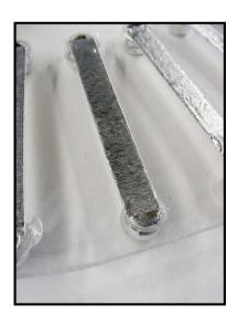
11. This figure shows the view from the other side of the disk. Each bead should be centered on the end of its foil strip. The corners of the strip *should not* protrude beyond the bead.
