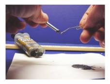
Mix up some metallic epoxy, often called "welding" epoxy, according to the instructions. If you absolutely can't find metallic epoxy, go ahead and use regular epoxy. With a paper clip, apply a dab of epoxy on each end. Allow the epoxy to cover the last 1/8th inch of the rod and form a small hemisphere at the end.
