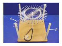
Then glue the legs (p) into the holes at the corners of the base. Slip the neutral support (e), *foil side down*, over two of the legs (p) as shown. The leg holes on the neutral support may be tight, so insert the legs gently to avoid cracking the neutral support. If the legs are too tight, you can
