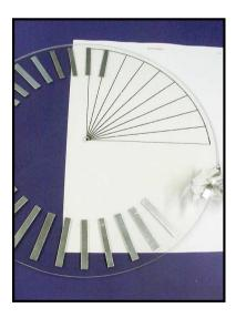
9. When you have applied about a quarter of the strips, rotate the disk and align the last few strips with the first few radial lines. Then continue adding strips until all of them have been applied. You should now have a disk with 36 equally-spaced foil strips.
