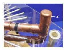
An endcap (x) goes on top of this pipe. Again, it should not be glued in place.
