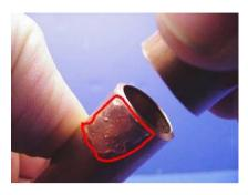
When attaching metal pipe to fittings, apply a thin layer of glue to one side of the pipe only. The other side should remain bare to provide electrical contact. A thin layer of glue may be applied to the outside once the fitting is in place. Soldering the fittings is neither necessary nor desirable.
