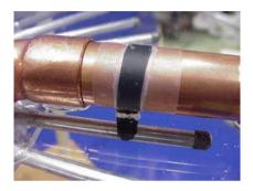
Tape each brush to a collector. I have used transparent tape so the brush can be seen, but you may use electrical tape. Replace the corona shield and adjust the leg sockets to ensure that the collector brushes make contact with each rod as the disk is turned. If the brushes are too short or too long, you may remove the tape and reposition them.
