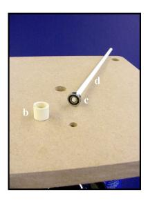
2. The main bearing is supported by a short length of half-inch CPVC tubing (b). Main bearing (c) is force-fit onto one end of the main shaft (d).
