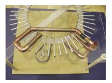
When both collectors and inductors have been assembled as shown, the corona shield can be Gooped to the leg sockets and the copper fittings can be tacked to the corona shield with spots of Goop. Slowly turning the disk by hand, confirm that each rod contacts a neutral brush as it passes beneath the inductor and a collector brush as it passes between the upper and lower collectors. When
