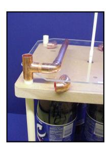
7. Remember, the four elbows underneath the corona shield are there only for support; do not glue them. Tubes (l) should be parallel to each other and to the sides of the corona shield. Allow the glue to set while you assemble the disk.
