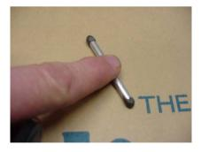
When the epoxy is no longer tacky, but still soft, roll each rod against a hard surface to remove any sagging.
