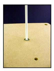
3. Apply some glue to bearing support (b) and insert it from *below*. into the hole in the center of base (a). The goal here is to avoid getting any glue on the bearing itself. Insert the bearing into the hole and adjust the bearing support until the bearing sits flush with the top of the base.
