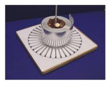
To make sure that glue contacts each rod, you will need to apply weight evenly to the disk. Use whatever you have at hand, but a roll of duct tape filled with pennies is perfect for the job.
