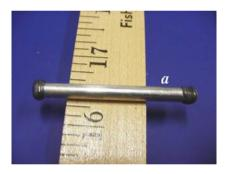
Place the rods (a) on a yardstick or ruler and allow the epoxy to set.
