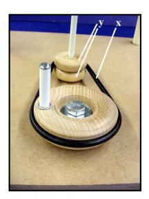
15. Force two small wooden wheels down the main shaft, almost to the main bearing. Separate the wheels slightly, apply glue between them, and force them back together. They should sit high enough above the main bearing that they do not touch the base. Slip the belt over the pulley and wheels to complete the drive section.
