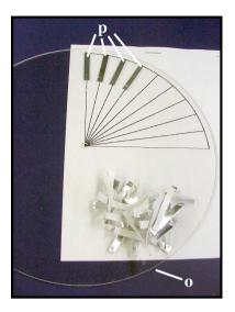
8. Peel the protective paper from the disk and place it over the disk template. Make sure that the hole in the disk is centered over the center of the template, as shown. Cut the adhesive foil tape into 36 strips (p), 2 inches long and 1/4 inch wide. Peel the protective paper from each foil strip and carefully stick it to the disk. Each strip should be centered on a radial line. Note that the foil strips *do not* go all the way to the edge of the disk.
