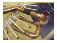
The inductor can now be inserted into the collector's 45 degree elbow (u). The inductor should sit directly over the neutral brush.
