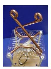
To use the big gap, remove the caps from the collector tees and slip the 45 degree elbows over the 1 inch pipes (z). Adjust the distance between the rods to about 1 inch and run the Dirod. Little by little, nudge the gap wider and wider until no spark leaps. Then move it back in for the biggest spark possible.
