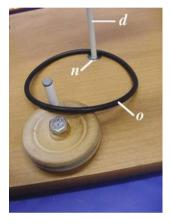
Place an end of the main axle (d) into the main bearing (n). Use a hammer to lightly force the axle into the bearing. The fit should be tight enough that no glue is needed. Place the bearing into the hole at the center of the base. Slip the belt (o) over the axle. When the Dirod is not in use, the belt should be left in this position so it doesn't stretch. When you want to run the Dirod, slip the belt over the pulley.
