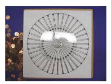
Make sure that the rods still line up with the template and that the center of the disk is lined up with the center of the template.
