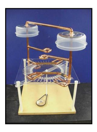
Dirod #7 is essentially a scaled-up Dirod #6 with enhancements to the inductors and collectors to reduce corona loss. Please read the Dirod #6 instructions before assembling Dirod #7. Only the differences between #6 and #7 will be given here.
