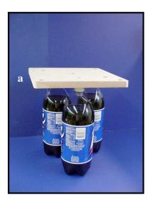
1. Because the legs will hang down below the base in the first phase of construction, you will need to elevate the base. I find that three 2-L soft-drink bottles are just the right size to support the base (a). The "front" of the generator has a small hole for the pulley. In addition to the holes at the corners and at the center, there are two 5/8-inch holes in the back-left and front-right corners.
